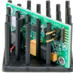
Thermobility Wireless Power Generator WPG-1
