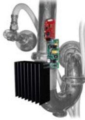
Clamp-on subsystem for harvesting energy from dispensed hot water
